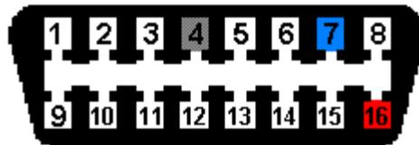
This is the socket-part, connector part is mirrored
