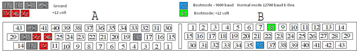
ECU connector: This is looking at the connector on the ECU
