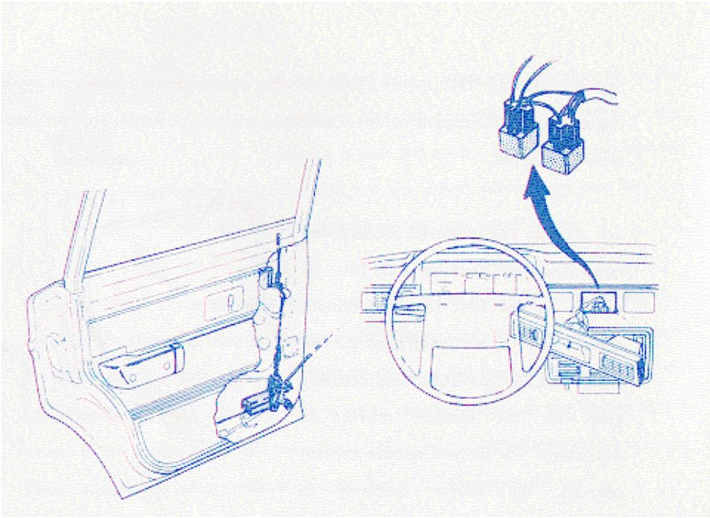
The top-of-the-line models in 1980 (GLE and 262 Coupe) also introduced other new or improved luxury features to Volvos. These included electrically operated door locks and an electronic cruise control instead of the mechanical system previously used. Typical replacement parts for the door locks system include the electric motor (usually one per door) and relays in the dashboard.
