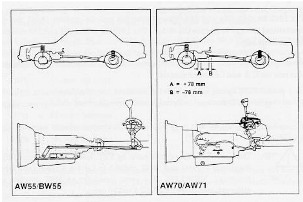
The AW70/71 transmissions are improved versions of the earlier automatics. The AW70 was fitted to normally aspirated (non-Turbo) four-cylinder sedans and wagons. The AW71 was fitted to all Turbo models equipped with automatic transmissions. The information plate on the side of the transmission and the VIC plate will positively identify the transmission.
