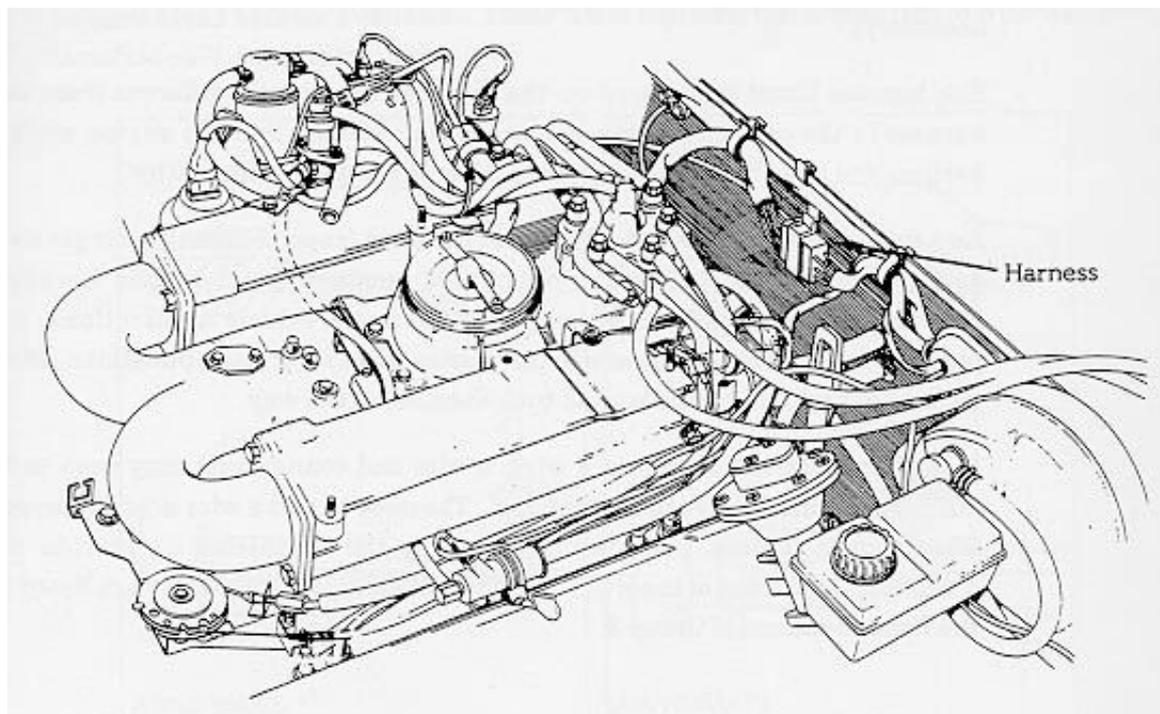
If a harness is needed, usually it's for a fire or accident-damaged car. There are many variations
