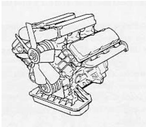
One last comment on the B-27 and B-28: the all-aluminum design make for a very lightweight engine. A genuine Volvo Exchange Program B-28F engine (if still available 10/98), tips the Parts Distribution Center scales at 290 lb. (132 kg). That's light when compared to some others:
