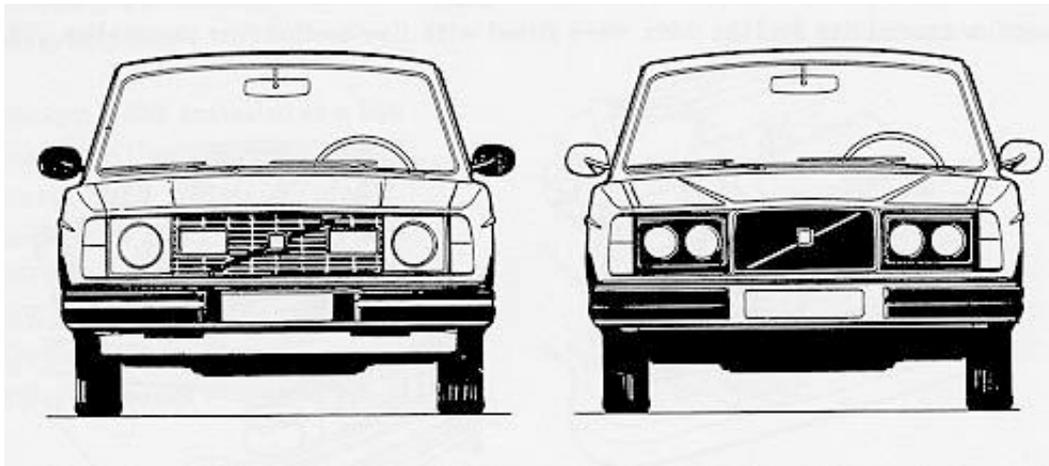
The headlamps were single round, dual round and dual rectangular headlight bulbs (the bulbs were called "inserts"). Although headlight inserts are listed by VIN on your Volvo Parts Manager's list, we have simplified things with the list below:
