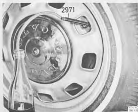
2971 Bleeder wrench for ATE-brakes
