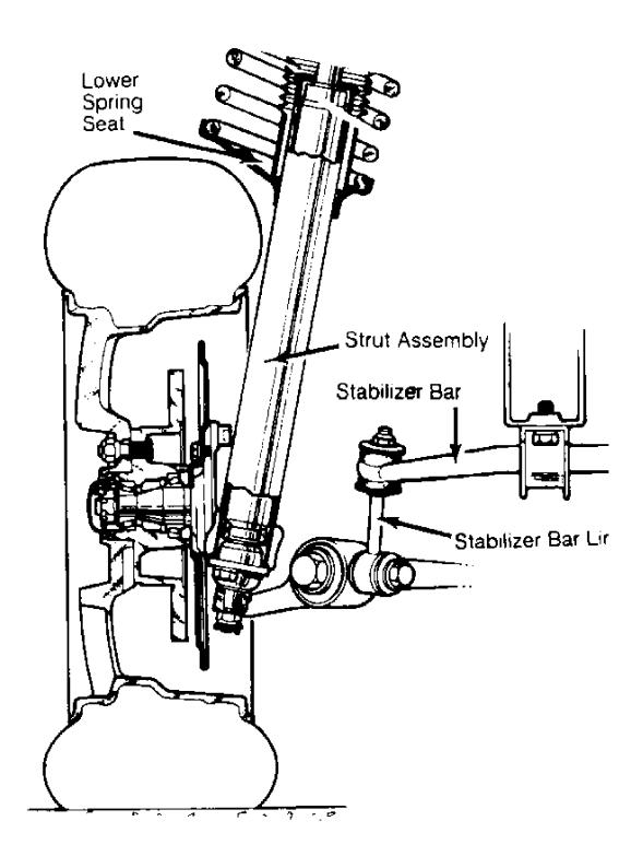
Fig. 2: Identifying Front Suspension Courtesy of Volvo Cars of North America
