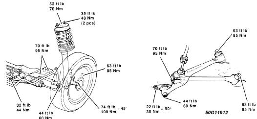
Fig. 3: Front Suspension Torque Specifications Courtesy of Volvo Cars of North America.
