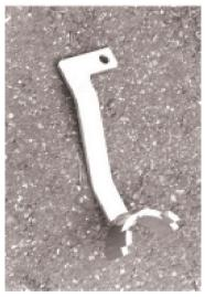
Volvo 5284 crankshaft pulley holder tool
