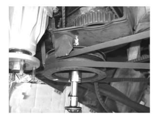
Figure 5. Use a 24 mm socket on the crankshaft bolt to rotate the crankshaft clockwise so as to . . .
