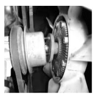
**Figure 1.** Take off the fan/clutch assembly by removing the 4 10-mm nuts. Pull assembly out.
