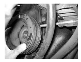
Figure 10. Without the belt tension, the crankshaft pulley should be easy to remove. Grab the pulley on opposite sides with both hands and rock it back and forth while pulling. If it is difficult to get off, gently pry in back with a flat-bladed screwdriver.
