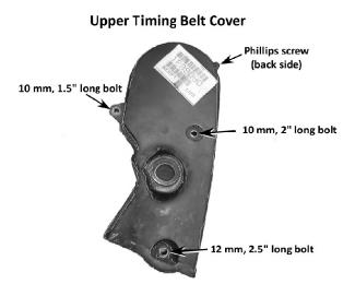
**Figure 3.** Remove all of the fasteners for the upper timing belt cover, as shown. During reassembly, this diagram will guide you as to which fastener goes where.
