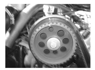
**Figure 6.** . . . align dot of overhead camshaft gear with nub on back timing belt plate.
