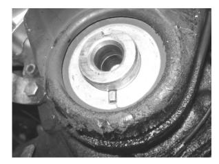
Figure 11. With the crankshaft pulley off, the front crankshaft shim and crankshaft end are exposed. (Note the oily residue at bottom of photo, which indicates a leaky crankshaft seal.)
