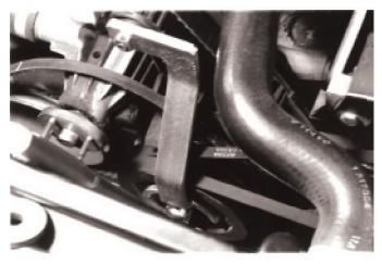
Volvo 5284 crankshaft pulley holder tool in use.
