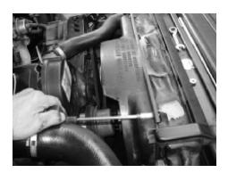
**Figure 2.** Remove the two 8-mm fasteners atop the fan shroud. Pull fan shroud out. Now you have more working room. (Some engines are different and may have more working room as a matter of design.)
