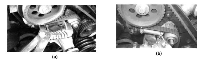
**Figure 13. (a)** Use a large pliers to squeeze the tensioner spring and insert a pin into the hole of the guide rod (b). Once the guide rod is pinned in place, compressing the spring, slip the old belt off. [If you are replacing the tensioner (**Appendix A**), pull that off now. Also, save old belt if you are replacing the oil seals. Why? See **Appendix B**.]
