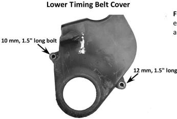
Figure 12. Remove the lower timing belt cover by extracting the 10 mm, 1.5" long bolt on the left and the 12 mm, 1.5" bolt on the right.
