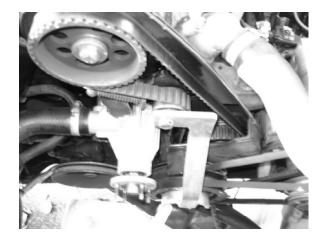
**Figure 7.** Remove the 17 mm nut and washer from the tensioner. Slip top of crankshaft pulley holder onto tensioner bolt, install the 17 mm nut, and finger tighten. Next, make sure the prongs on the bottom of holder catches the holes in the crankshaft gear/vibration dampener (hereafter called just crankshaft gear or pulley), turning the crankshaft with the 24 mm socket, if needed. Once the prongs catch, tighten the 17 mm nut on the tensioner.
