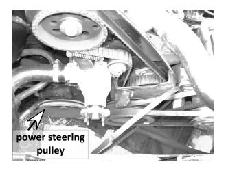
**Figure 4.** Upper timing belt cover removed. Note waterpump/power steering belt hanging over the alternator and air conditioning compressor belts. (Arrow shows power steering pulley.)
