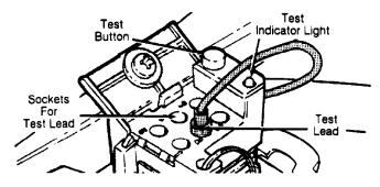
Fig. 7: Identifying Diagnostic Unit Components Courtesy of Volvo Cars of North America.
