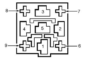
93G78481 Fig. 4: Identifying Fuel Pump Relay Terminals (850) Courtesy of Volvo Cars of North America.
