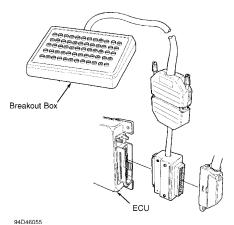
Fig. 6: Connecting Breakout Box To ECU (960 Shown; 850 Is Similar) Courtesy of Volvo Cars of North America. Injection System (Fuel Pump) Relay (940)
