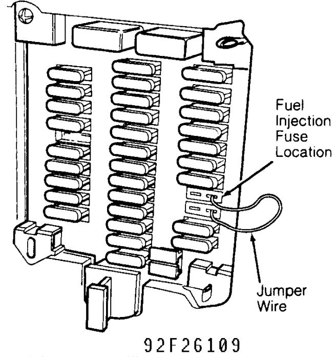
Fig. 5: Identifying Fuel Pump Fuses (960) Courtesy of Volvo Cars of North America.
