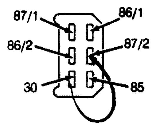
Fig. 3: Identifying Fuel Injection System Relay Terminals (940) Courtesy of Volvo Cars of North America.
