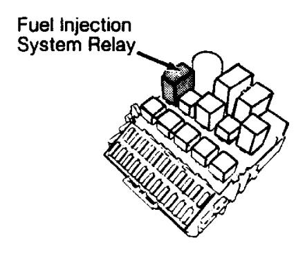
Fig. 1: Locating Fuel System Relay (940) Courtesy of Volvo Cars of North America.
