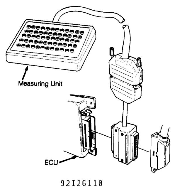
Fig. 3: Connecting Measuring Unit (999-3070) To ECU Courtesy of Volvo Cars of North America.
