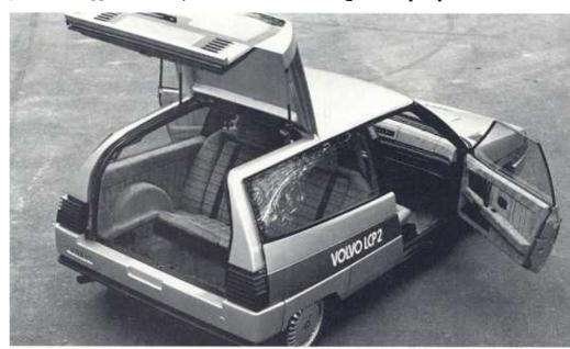
of fiber reinforced nylon. Carbon fiber has been used to make graceful and extremely light door glass frames. In fact, although cast iron and steel were used for driveshafts, gears and other highly stressed components, only about 320 pounds of the car's total weight is from such conventional automotive materials.
