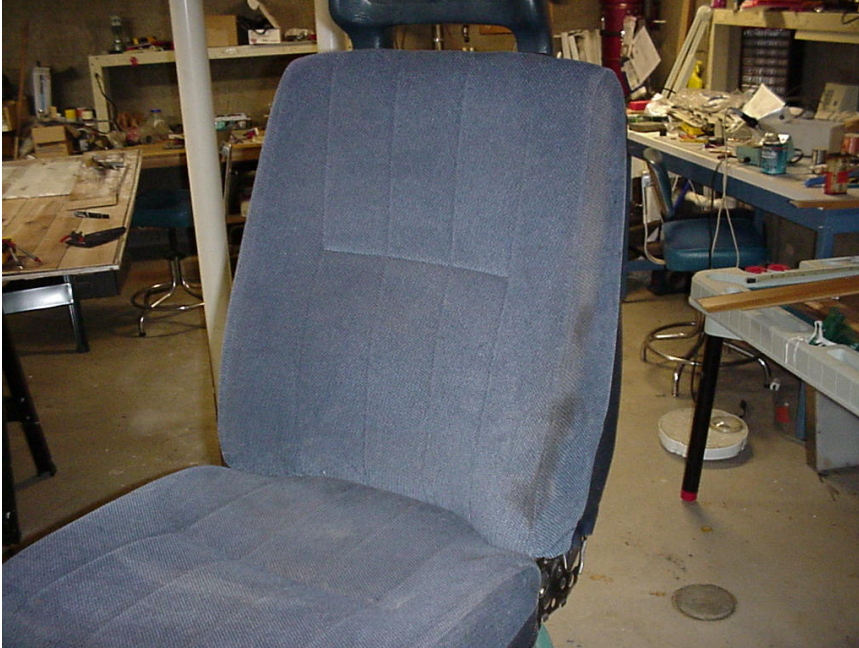
C. donor seat, grease on seat and holes in the cloth but foam is excellent out of a '92 245.
