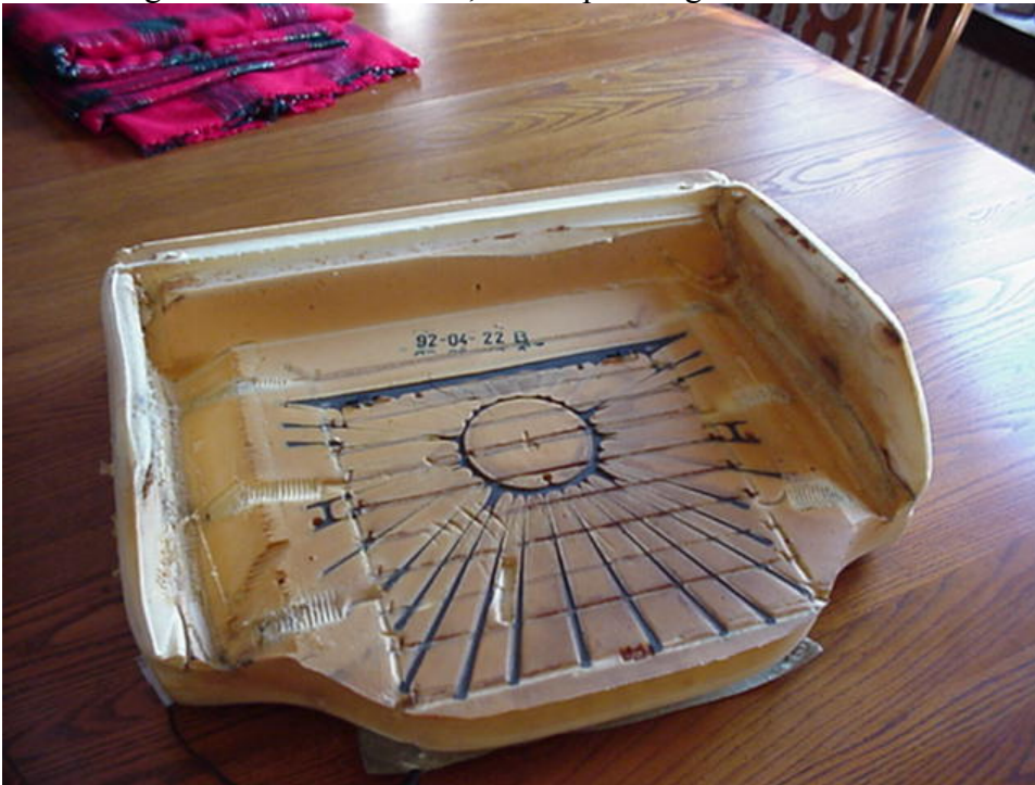
P. Size of patch to put on each side. Smaller patch is used at the tear area then this larger one is applied over it. The patches I used was call Batting from an upholsterer. He gave
