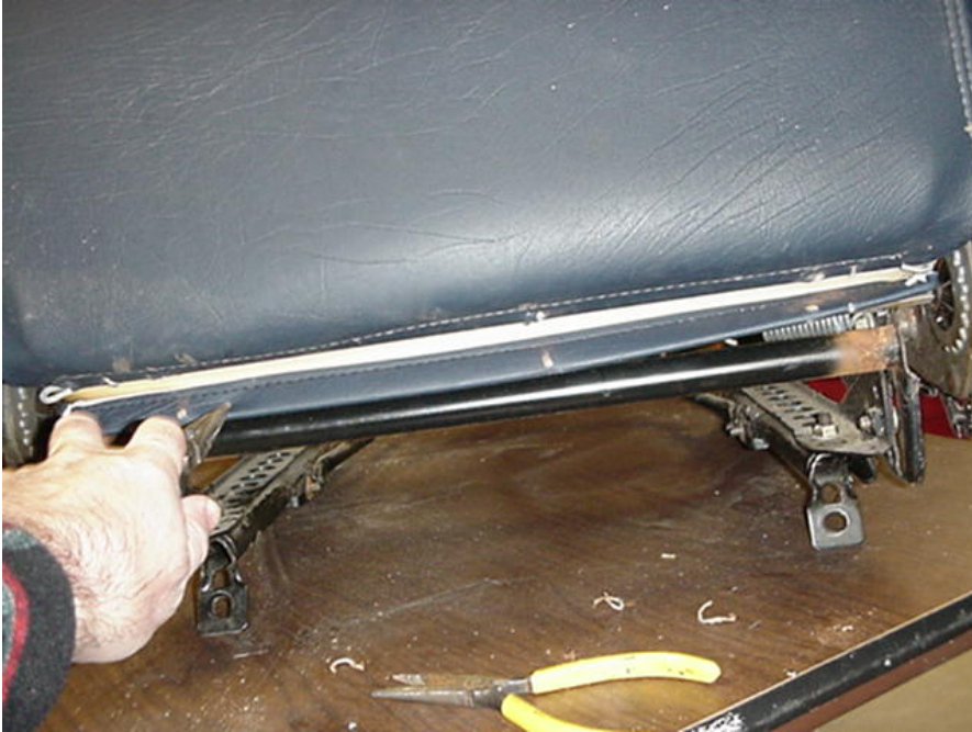
G. The second set holds the back part of the cover to the steel frame
