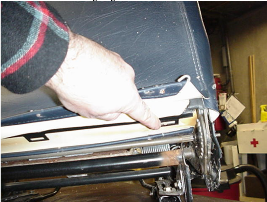
H. Shows where the Hog rings hold to frame.
