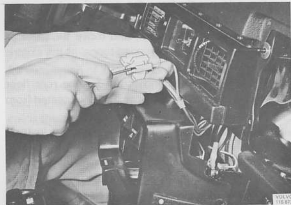
Removing electric cables for contact unit
