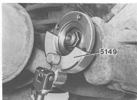
5149 Wrench installing/removing drive flange
