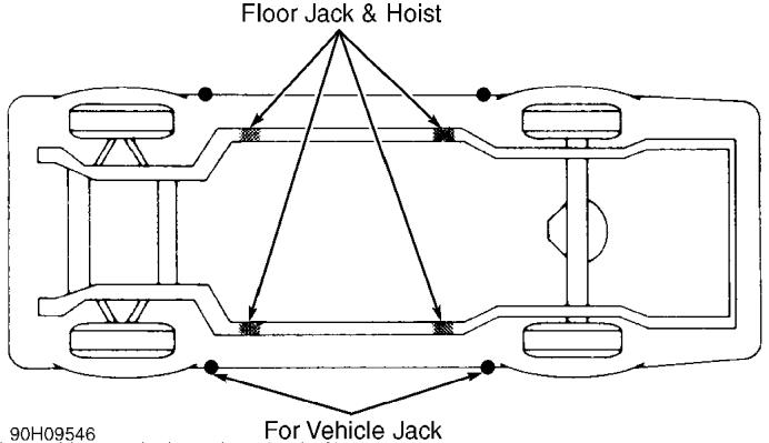
Fig. 1: Jacking & Hoisting Points (Typical)
