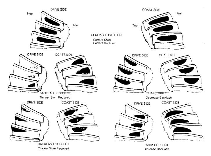
Fig. 1: Drive Axle Gear Tooth Patterns
