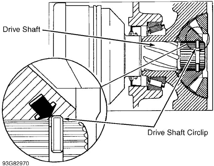
Fig. 1: Installing Left Drive Shaft Courtesy of Volvo Cars of North America
