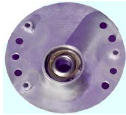
Top View 'offset centre' left hand strut bearing mounts GpA Underside View -2 to -4 deg
