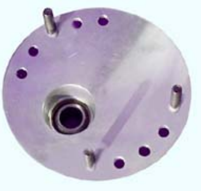
Top View 'offset centre' left hand strut bearing mounts GpA Underside View -2 to -4 deg
